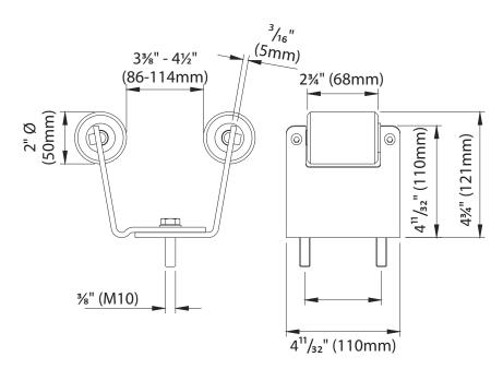
The gate receiver can be installed on the closed side of the gate to keep the gate steady at the top. Install the gate receiver to a mounting bracket.
