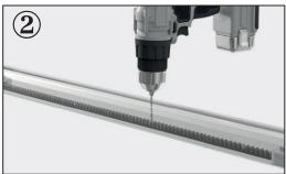
Using the pre-drilled gear rack as a guide, drill mounting holes in the track. Screw the gear rack to the track.
