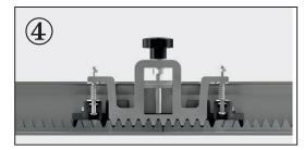
Position the template guide between two pieces of gear rack and tighten the locking screw. The gear rack teeth are registered and spaced correctly as the guide is tightened into place. After locking the second guide at the far end of the gear rack, use the pre-drilled gear rack as a guide to continue drilling mounting holes in the track.
