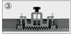
Insert the second piece of gear rack.
