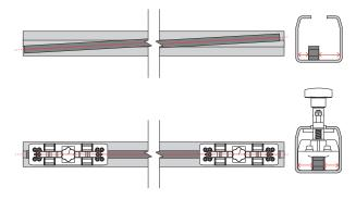
Position the first piece of gear rack inside the track. Use two template guides, one positioned at each end of the gear rack to center the gear rack lengthways within the track.
