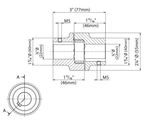
USE: Adapter for connecting Integrator carriages with motor. TYPE: Adapter for Piccolo and Mini Integrator carriages. FIXING: Use 2 M6 headless screws.
