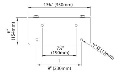
USE: Guide plate for sliding gates and self-supporting. TYPE: Adjustable gate guide plate with long leaf for fixing. FIXING: For fixing.
