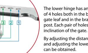
The lower hinge has an adjustment system consisting of 4 holes both in the bracket that connects to the gate leaf and in the bracket that connects to the post. Each pair of holes (1, 2, 3, 4) corresponds to an inclination of the gate.
