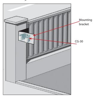
${\sf USE: Adjustable\ striker\ plate\ for\ sliding\ or\ self-supporting\ gates.}$
