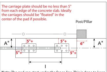
Note: The pad can start under the fence line. This is done to keep the gate face at no more than 2-1/4" from the fence line and to avoid entrapment.
