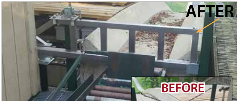
DuraGates installed at a toboggan park. The gate removes the cumbersome task of removing the chain for each rider.
